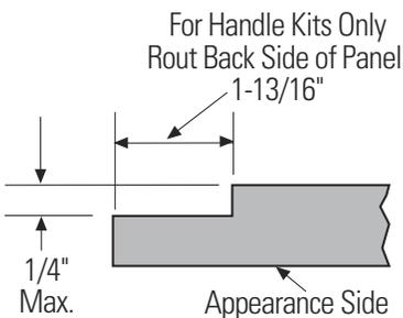
Route the panel when installing a ZKHTR1 Custom Handle Kit or ZKHTRSS1, Tubular Stainless Steel Handle Kit.
