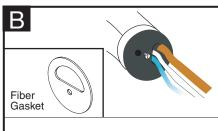
Make sure to use fiber gasket to ensure proper seal.
